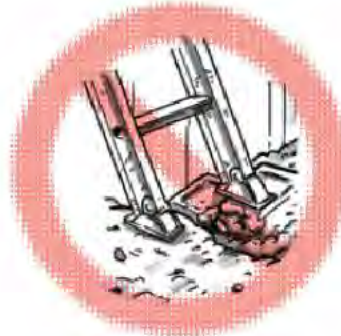
DON'T place the ladder on unlevel footing
