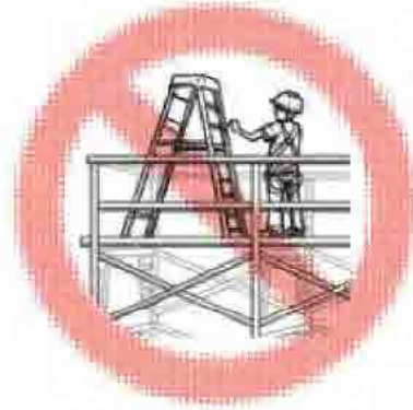
DON'T use a ladder on top of a scaffold
